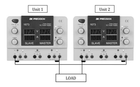
Figure 7 - Connecting Multiple Units in Series
