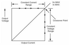
Figure 4 - CC/CV Characteristic
