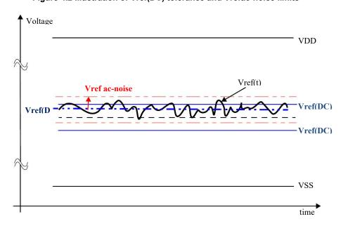
Figure 4.2 Illustration of Vref(DC) tolerance and Vrefac-noise limits
