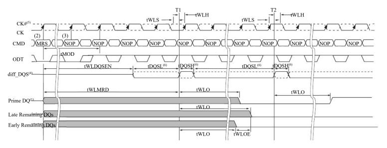
Figure 2.4.7.2 Write leveling sequence [DQS - DQS# is capturing CK-CK# low at T1 and CK-CK# high at T2]
