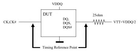
Figure 5.5 Reference Load for AC Timing and Output Slew Rate
