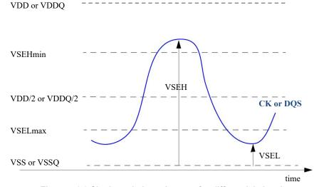
Figure 4.3.3 Single-ended requirement for differential signals.
