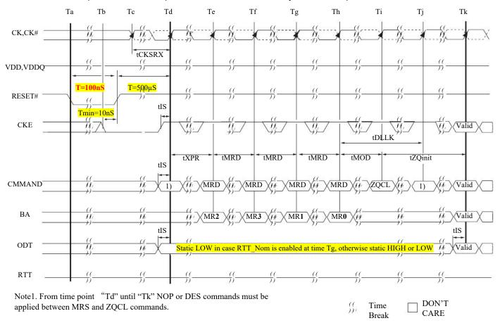
Figure 2.1.2 Reset Procedure at Power Stable Condition
