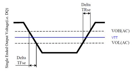
Figure 5.3.1 Single Ended Output Slew Rate Definition
