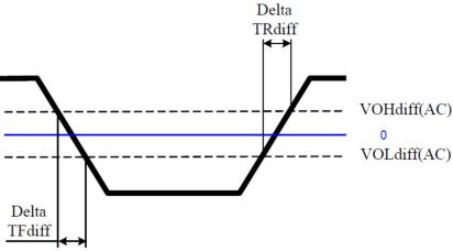
Figure 5.4.1 Differential Output Slew Rate Definition
