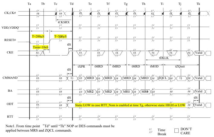
Figure 2.1.1 Reset and Initialization Sequence at Power-on Ramping
