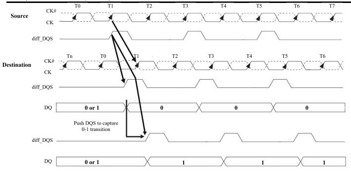
Figure 2.4.7 Write Leveling Concept
