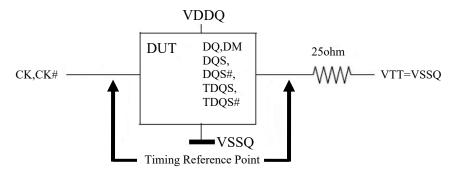
Figure 5.9.1 ODT Timing Reference Load
