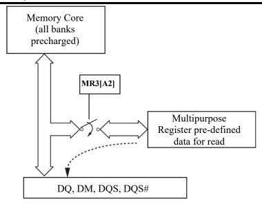
Figure 2.3.5.1 MPR Block Diagram
