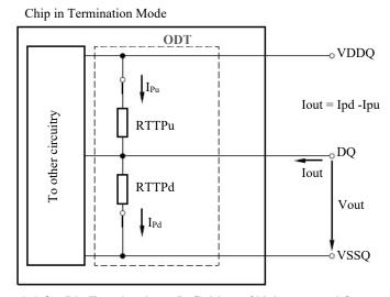
Figure 5.8.1 On-Die Termination : Definition of Voltages and Currents
