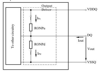
Figure 5.7 Output Driver: Definition of Voltages and Currents
