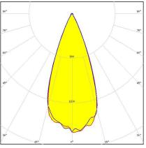
Dimensions: 35.0 mm x 35.0 mm Height: 15.00 mm ~40° beam
