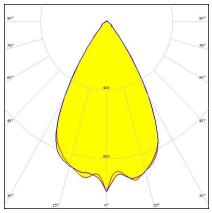
Dimensions: 35.0 mm x 35.0 mm Height: 13.42 mm ~60° beam
