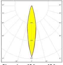
Dimensions: 35.0 mm x 35.0 mm Height: 14.52 mm ~20° beam
