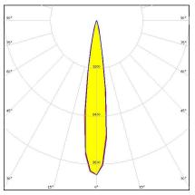
**Dimensions: 21.6 mm x 21.6 mm Height: 13.10 mm** ~8° spot beam. Assembly with thinner white holder, installation tape and location pins.
