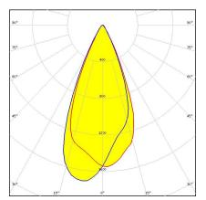
**Dimensions: 21.6 mm x 21.6 mm Height: 13.10 mm** ~40° wide beam optimized for CREE XP-E. Assembly with white holder, installation tape and location pins.
