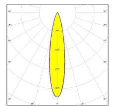
Dimensions: 21.6 mm x 21.6 mm Height: 13.10 mm ~13° diffused spot beam. Assembly with thinner white holder installation
