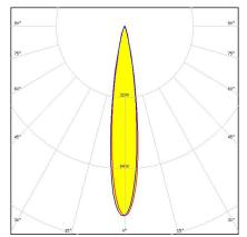
Dimensions: 21.6 mm x 21.6 mm Height: 13.10 mm ~11° smooth spot beam. Assembly
