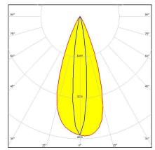
**Dimensions: 21.6 mm x 21.6 mm Height: 13.10 mm** ~40° x 13° oval beam. Assembly with thinner white holder, installation tape and location pins.
