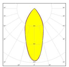
Dimensions: 21.6 mm x 21.6 mm Height: 13.10 mm ~65° wide beam. Assembly with thinner white holder, installation tape and location pins.
