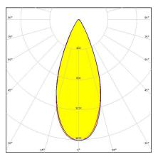
**Dimensions: 21.6 mm x 21.6 mm Height: 13.10 mm** ~45° wide beam. Assembly with thinner white holder, installation tape and location pins.
