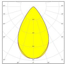
Dimensions: 21.6 mm x 21.6 mm Height: 13.10 mm ~65° wide beam optimized for CREE XP-E. Assembly with black holder and installation tape.
