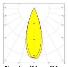
Dimensions: 30.0 mm x 30.0 mm Height: 18.45 mm ~40° wide beam with flange
