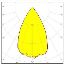
Dimensions: 30.0 mm x 30.0 mm Height: 18.45 mm ~60° wide beam with flange.
