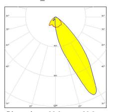
Dimensions: 32.0 mm x 32.0 mm Height: 20.75 mm Asymmetric beam for wall-washing.
