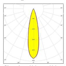
Dimensions: 30.0 mm x 30.0 mm Height: 18.45 mm ~11° spot beam with flange
