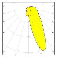
Dimensions: 53.9 mm x 53.9 mm Height: 24.65 mm Asymmetric beam for wall washing with holder C compatible with LEDiL
