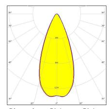
Dimensions: 52.1 mm x 52.1 mm Height: 16.98 mm ~45° wide beam with holder C
