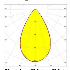
Dimensions: 69.9 mm x 69.9 mm Height: 14.60 mm ~60° wide beam with holder B
