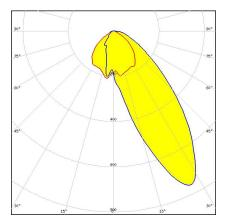
Dimensions: 69.9 mm x 69.9 mm Height: 14.60 mm Asymmetric beam for wall-washing with holder A compatible with TE,
