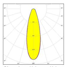
Dimensions: 69.9 mm x 69.9 mm Height: 17.20 mm ~25° spot beam with holder A
