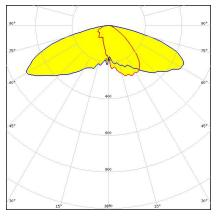
Dimensions: 18.0 mm x 18.0 mm Height: 7.70 mm IESNA Type II (medium) beam,
