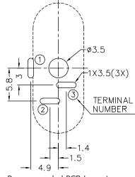
Recommended PCB Layout Top View
