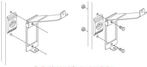
**Padlocking Lock System Installation**
