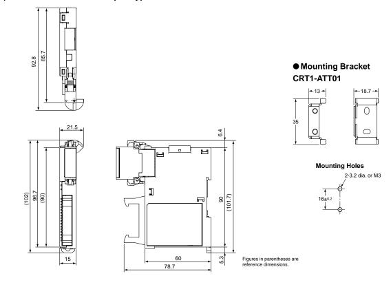
Digital I/O Slave Units with MIL Connector (Vertical type)
