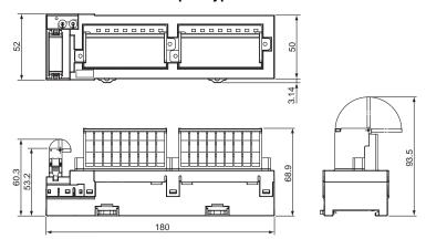
Digital I/O Slave Units with e-CON Connectors
