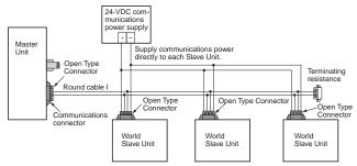
Before connecting the power supply, first connect a DCN4-TB4 Open Type Connector to the communications connector to convert it to a screw terminal block
