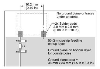
Figure 11. uSP410 Series Antenna Placement on PCB.
