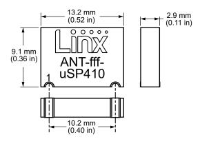
Figure 6. uSP410 Series Antenna Dimensions
