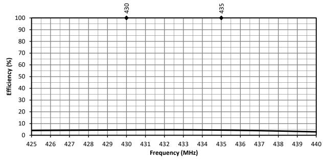
Figure 5. ANT-433-uSP410 Radiation Efficiency
