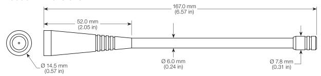
Figure 6. CW 450 MHz Antenna Dimensions
