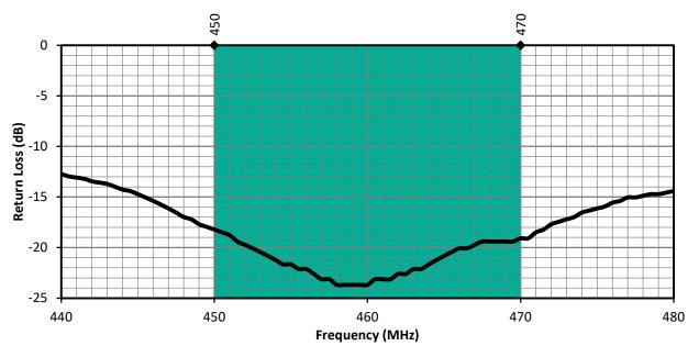
Figure 2. CW 450 MHz Antenna Return Loss with Band Highlight
