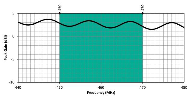
Figure 3. CW 450 MHz Antenna Peak Gain with Band Highlight
