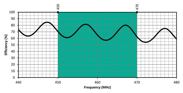
Figure 5. CW 450 MHz Antenna Radiation Efficiency with Band Highlight
