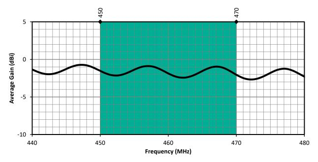
Figure 4. CW 450 MHz Antenna Average Gain with Band Highlight
