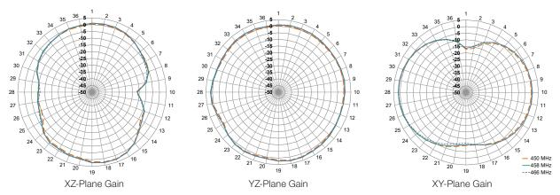
Figure 8. Radiation Patterns for CW 450 MHz Antenna
