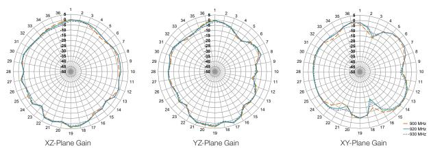
Figure 7. ANT-8/9-VDP-2000 Radiation Patterns
