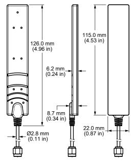
Figure 1. ANT-8/9-VDP-2000 Antenna Dimensions
