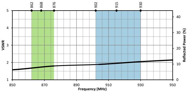
Figure 2. ANT- 8/9-VDP-2000 VSWR with Frequency Band Highlights
