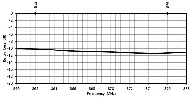
Figure 4. ANT-868-CW-RCL Return Loss
