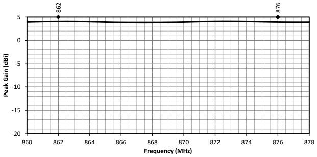
Figure 5. ANT-868-CW-RCL Peak Gain
