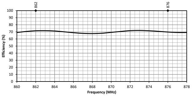
Figure 7. ANT-868-CW-RCL Antenna Radiation Efficiency
