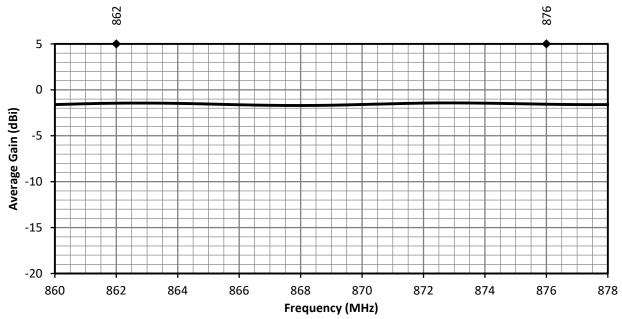
Figure 6. ANT-868-CW-RCL Antenna Average Gain
