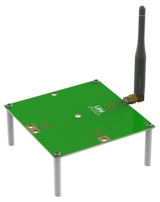
Figure 2. ANT-868-CW-RCL on Evaluation PCB
