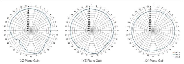
Figure 8. ANT-868-CW-RCL Radiation Patterns
