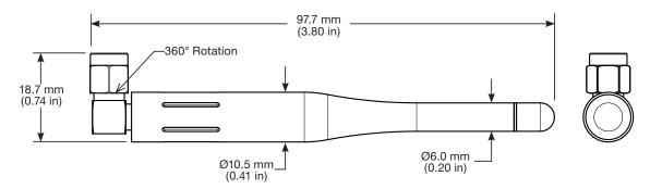
Figure 1. ANT-868-CW-RCL Antenna Dimensions
