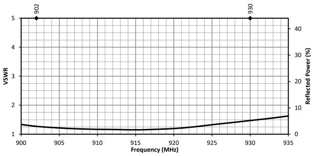
Figure 12. ANT-916-WRT VSWR, Center of Ground Plane
