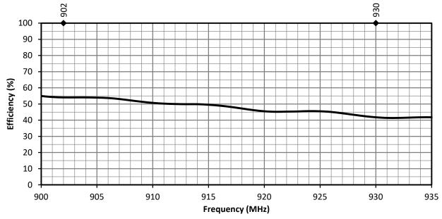
Figure 9. ANT-916-WRT Antenna Radiation Efficiency, Free Space
