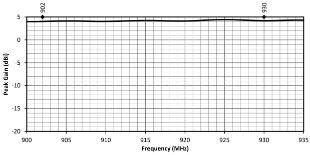
Figure 14. ANT-916-WRT Peak Gain, Center of Ground Plane
