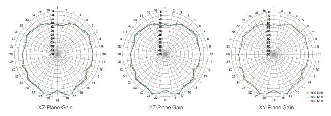
Figure 17. ANT-916-WRT Radiation Patterns, Center of Ground Plane
