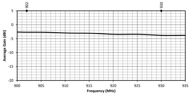
Figure 8. ANT-916-WRT Antenna Average Gain, Free Space
