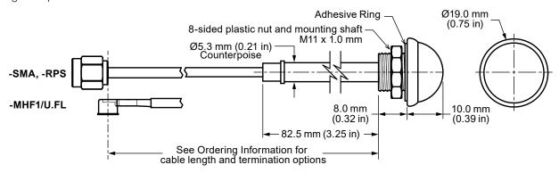
Figure 1. ANT-916-WRT Antenna Dimensions
