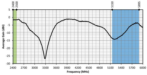
Figure 7. ANT-DB1-WRT-MON Antenna Average Gain, with Frequency Band Highlights
