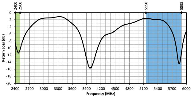
Figure 5. ANT-DB1-WRT-MON Return Loss, with Frequency Band Highlights
