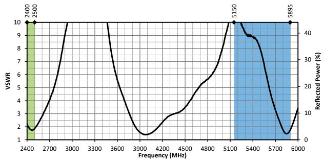
Figure 4. ANT-DB1-WRT-MON VSWR, with Frequency Band Highlights
