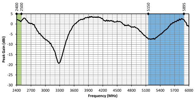
Figure 6. ANT-DB1-WRT-MON Peak Gain, with Frequency Band Highlights
