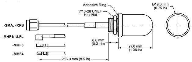
Figure 1. ANT-DB1-WRT-MON Antenna Dimensions
