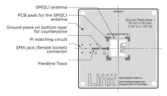
Figure 9. GNSSCP-SM12L1 Recommended Layout
