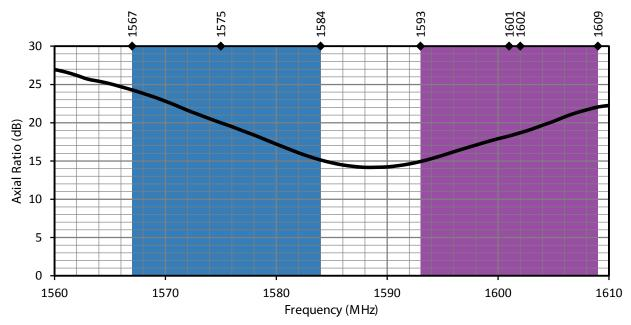
Figure 6. GNSSCP-SM12L1 Antenna Axial Ratio
