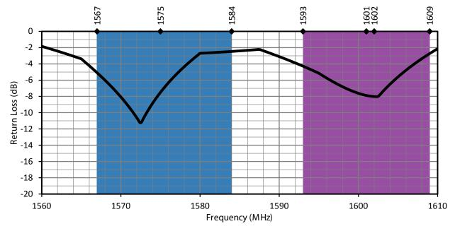
Figure 3. GNSSCP-SM12L1 Return Loss
