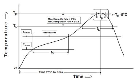
Figure 12. Solder Profile for the GNSSCP-SM12L1 Antenna
