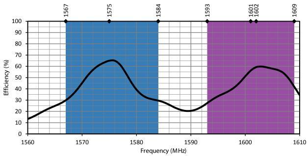
Figure 7. GNSSCP-SM12L1 Antenna Radiation Efficiency
