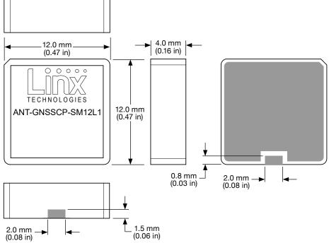
Figure 1. GNSSCP-SM12L1 Antenna Dimensions
