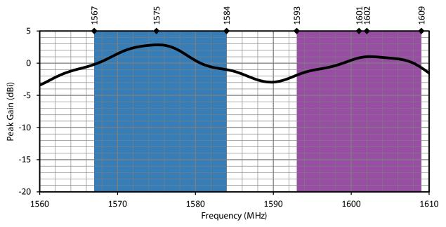
Figure 4. GNSSCP-SM12L1 Peak Gain
