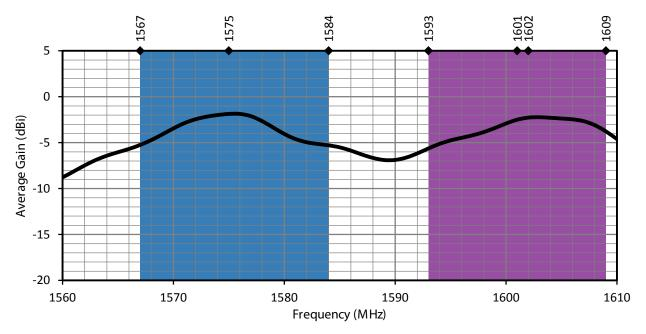
Figure 5. GNSSCP-SM12L1 Antenna Average Gain
