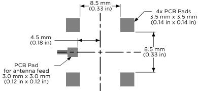
Figure 11. ANT-GNSSCP-SM12L1 Antenna Placement on PCB
