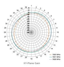
Figure 8. ANT-GNSSCP-SM12L1 Radiation Patterns
