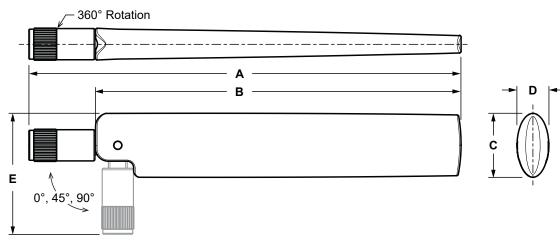
Figure 1. W63WSx Series Antenna Dimensions
