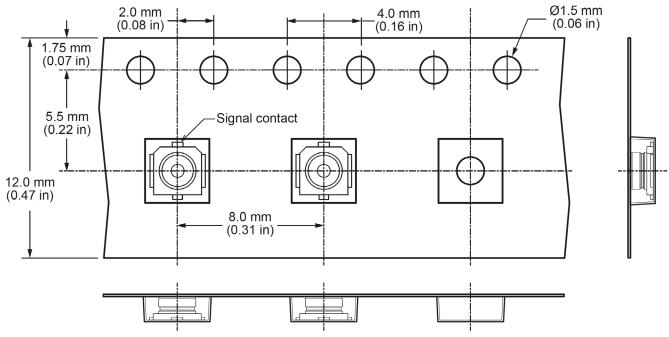
Figure 4. Tape Specifications for the CONMHF1-SMD Connector
