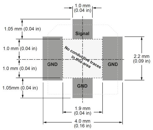
Figure 2. Recommended PCB Dimensions for the CONMHF1-SMD
