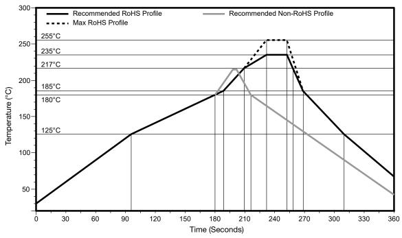
Figure 3. CONMHF1-SMD Recommended Reflow Solder Profile
