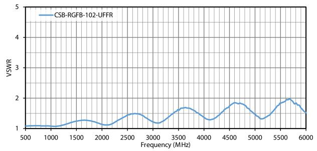
Figure 5. VSWR for the CSB-RGFB-102-UFFR Cable Assembly
