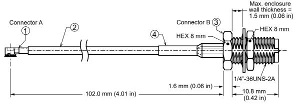
Figure 1. Product Dimensions for the CSB-RGFB-102-UFFR Cable Assembly
