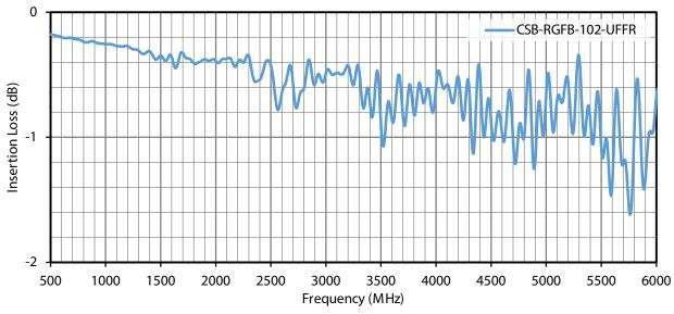
Figure 4. Insertion Loss for the CSB-RGFB-102-UFFR Cable Assembly
