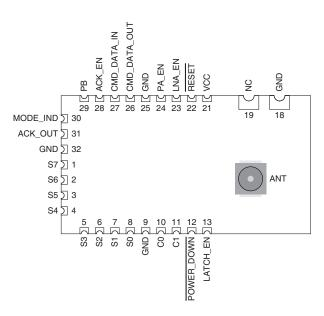
Figure 15: HumPRC<sup>™</sup> Series Transceiver Encapsulated Version Pin Assignments - UFL Connection (Top View)
