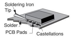
Figure 95: Soldering Technique
