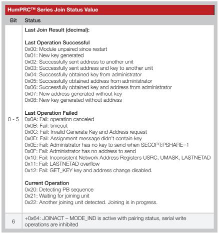
Figure 77: HumPRC™ Series Transceiver Join Status Value
