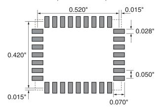
Figure 90: HUM-\*\*\*-PRC Recommended PCB Layout
