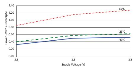
Figure 11: HumPRC™ Series Transceiver Standby Current Consumption vs. Supply Voltage
