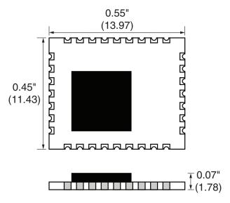
Figure 17: HumPRC™ Series Transceiver Dimensions
