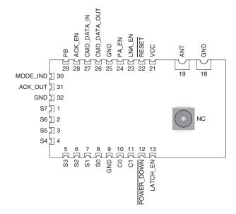
Figure 13: HumPRC™ Series Transceiver Encapsulated Version Pin Assignments - Castellation Connection (Top View)
