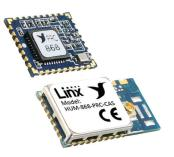
The module provides long-range transmission at 868MHz utilizing Listen Before Talk and
