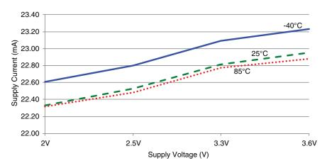
Figure 9: HumPRC™ Series Transceiver TX Current vs. Supply Voltage at 0dBm
