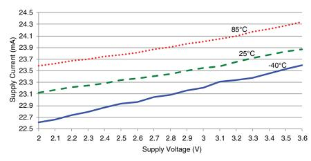
Figure 10: HumPRC™ Series Transceiver RX Scan Current vs. Supply Voltage, 38.8kbps
