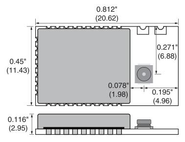
Figure 18: HumPRC<sup>™</sup> Series Transceiver Encapsulated Version Dimensions
