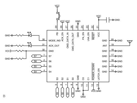
Figure 84: HumPRC™ Series Transceiver Basic Application Circuits for Remote Control
