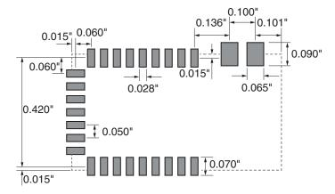
Figure 91: HUM-\*\*\*-PRC-UFL/CAS Recommended PCB Layout
