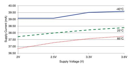
Figure 7: HumPRC™ Series Transceiver TX Current vs. Supply Voltage at Max Power
