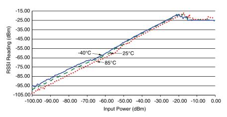
Figure 12: HumPRC™ Series Transceiver RSSI Voltage vs. Input Power
