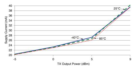
Figure 8: HumPRC™ Series Transceiver Average TX Current vs. Transmitter Output Power at 3.3V
