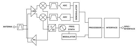
Figure 19: HumPRC™ Series Transceiver RF Section Block Diagram
