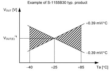
\*1.  $V_{OUT(E)}$  is the value of the output voltage measured at Ta = +25°C.
