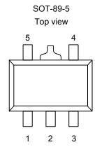
Pin No. Symbol Description ON/OFF 1 ON/OFF pin 2 VSS GND pin NC<sup>\*1</sup> 3 No connection VIN 4 Input voltage pin 5 VOUT Output voltage pin
