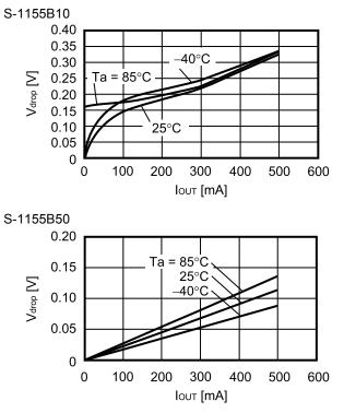
4. Dropout Voltage vs. Set Output Voltage
