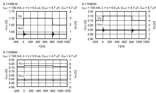
2. Characteristics of Load Transient Response (Ta = 25°C)
