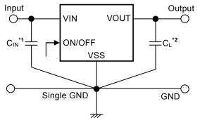
**\*1.**  $C_{IN}$  is a capacitor for stabilizing the input.
