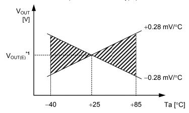
\*1.  $V_{OUT(E)}$  is the value of the output voltage measured at Ta = +25°C.
