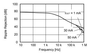
S-1165B30 (Ta = 25°C)  $V_{IN} = 4.0 \text{ V, Cout} = 2.2 \mu F$
