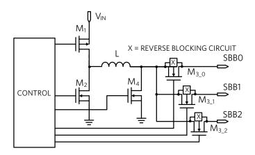
Figure 7. SIMO Power Block Diagram
