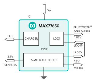
Figure 5. MAX77650 Highly Integrated PMIC
