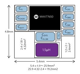
Figure 9. MAX77650 Solution (19.2mm<sup>2</sup>)
