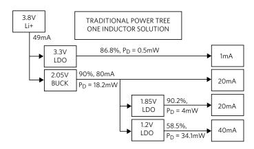
Figure 3. Typical Hearable Power Flow Diagram
