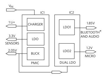
Figure 2. Typical Hearable Power Flow Diagram
