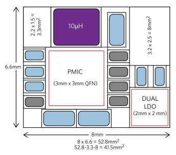
Figure 4. Typical Hearable Solution (41.5mm<sup>2</sup>)
