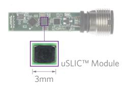
Figure 7. MAXM17532 in a tiny proximity sensor
