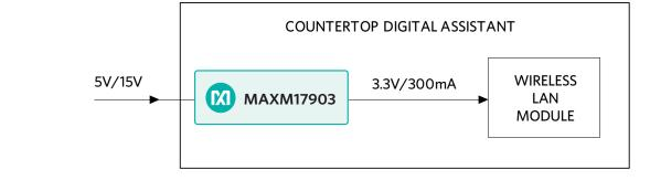
Figure 13. MAXM17903 uSLIC powering wireless LAN module
