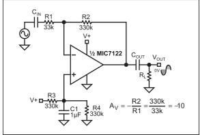
FIGURE 3-8: AC-Coupled Inverting Amplifier.
