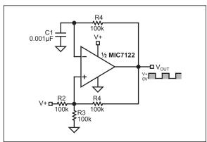
FIGURE 3-7: Square Wave Oscillator.
