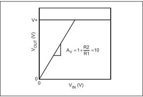
FIGURE 3-4: Non-Inverting Amplifier Behavior.
