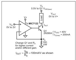
FIGURE 3-6: Voltage-Controlled Current Sink.
