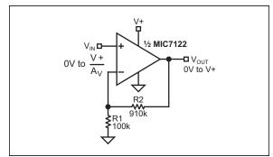
FIGURE 3-3: Non-Inverting Amplifier.
