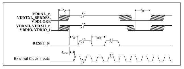
The recommended power-up sequence is to have the transceiver (VDDAH, VDDAH\_x) and digital I/O (VDDIO, VDDIO\_1) voltages power up before the 1.1V core (VDDCORE, VDDAL\_x, VDDTXL\_SERDES) voltage. If the 1.1V core must power up first, the maximum lead time for the 1.1V core voltage with respect to the transceiver and digital I/O voltages must be 200 µs.
