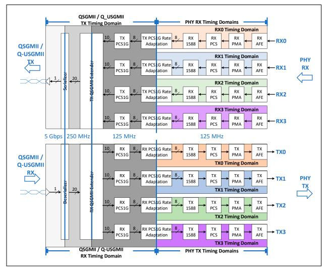
FIGURE 5-13: QSGMII/Q-USGMII SYSTEM DIAGRAM
