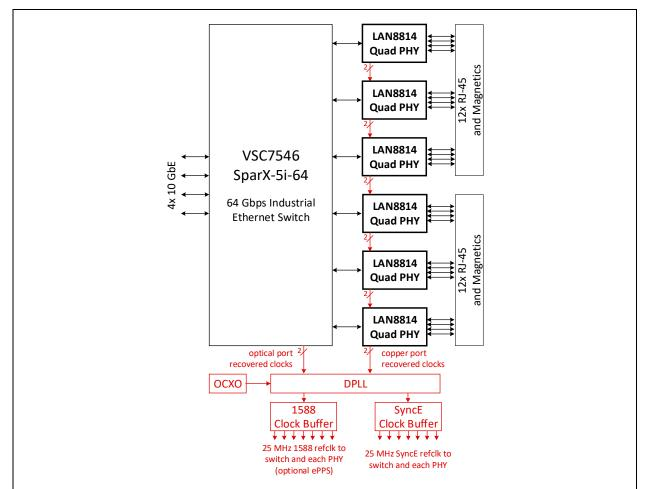
FIGURE 5-2: SYNCHRONOUS ETHERNET AND IEEE 1588 SYSTEM DIAGRAM
