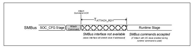
TABLE 9-8: USB ATTACH COMMAND TO SMBUS SLAVE READY TIMING
