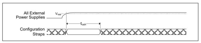
TABLE 9-5: POWER-ON CONFIGURATION STRAP LATCHING TIMING
