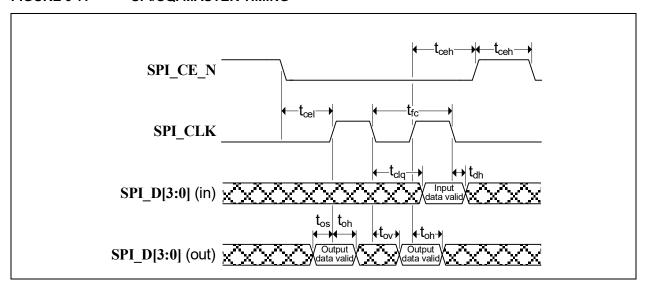
TABLE 9-9: SPI/SQI MASTER TIMING (30 MHZ OPERATION)
