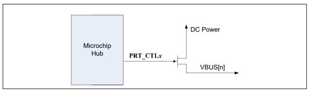
If the OEM provides an external supply capable of supplying current per the battery charging specification, the hub can be configured to indicate the presence of such a supply from the device. This indication, via the PRT\_CTLx pins, is on a per port basis. For example, the OEM can configure two ports to support battery charging through high current power FETs and leave the other two ports as standard USB ports.
