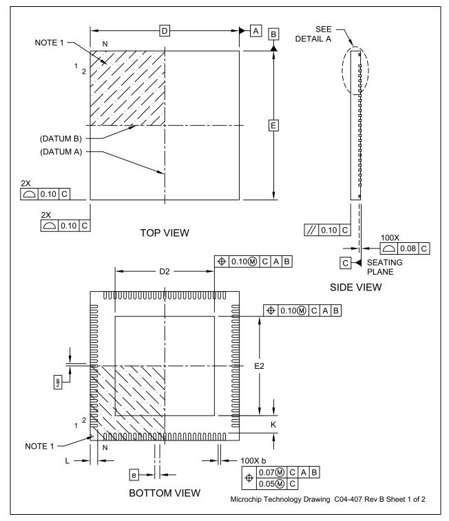
FIGURE 10-2: 100-VQFN PACKAGE (DIMENSIONS)
