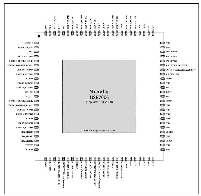
**Note:** Configuration straps are identified by an underlined symbol name. Signals that function as configuration straps must be augmented with an external resistor when connected to a load.
