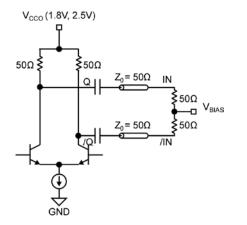
Figure 5c. CML AC-Coupled Termination.
