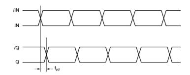
Figure 1. Propagation Delay
