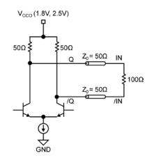
Figure 5b. 1.8V, 2.5V CML DC-Coupled Termination
