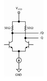
Figure 2b. Simplified CML Output Buffer
