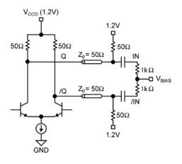
Figure 5d. CML AC-Coupled Termination.
