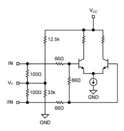
Figure 2a. Simplified Differential Input Buffer
