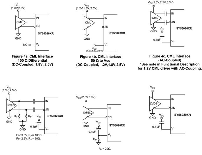
Figure 4d. LVPECL Interface (AC-Coupled)
