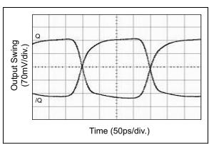
FIGURE 2-2: 2.5 GHz Output.
