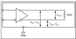
FIGURE 8-1: LVDS Differential Measurement.
