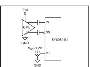
FIGURE 7-2: CML Interface (AC-Coupled).
