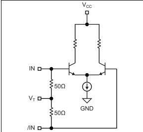
FIGURE 6-1: Simplified Differential Input Stage.
