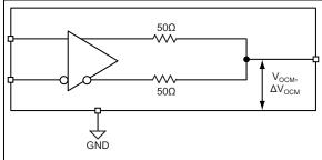
FIGURE 8-2: LVDS Common Mode Measurement.
