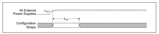
TABLE 9-5: POWER-ON CONFIGURATION STRAP LATCHING TIMING
