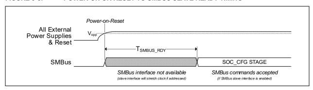
TABLE 9-7: POWER-ON OR RESET TO SMBUS SLAVE READY TIMING
