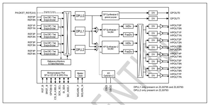
Figure 1 - Functional Block Diagram
