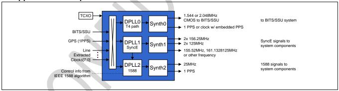
Figure 2 - Synchronous Ethernet and IEEE 1588 Central Timing Application
