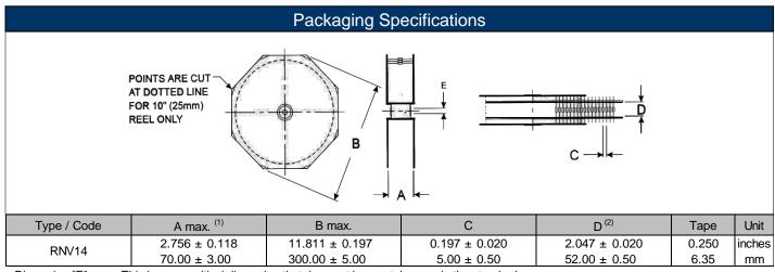
Dimension "E": This is a non-critical dimension that does not have a tolerance in the standard. Range of diameters is from 0.547" (13.9 mm) to 1.5" (38.1 mm)
