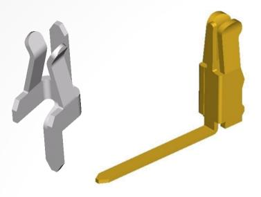
M20 and M22 sockets feature dual beam contacts, typically in phosphor bronze or other high-quality spring material. The dual beam connection gives good durability, repeatable retention and a reliable connection, offering a dependable, cost-effective connector. Design types include flat beam designs (as shown above) and tuning fork designs.
