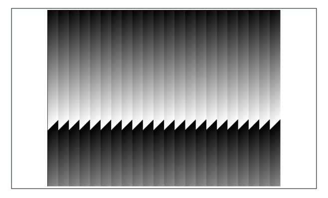
In sub-LVDS test mode 3, the actual data of every pixel is replaced by the output of a pseudo-random generator. The value of the first valid pixel of a frame is 4095. All outputs drive the same output value (unlike test mode 2, where the  $N_{\text{KERNEL}}$  generates an offset between outputs).
