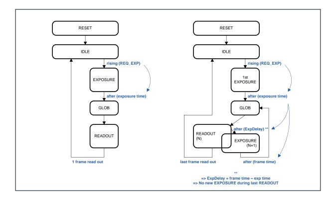
When exiting IDLE mode, the behavior is identical to Programmed External mode: a rising edge on REQ\_EXP will initiate the EXPOSURE state, which ends after a register defined exposure time. When the exposure time expires, a GLOB state is started, followed by READOUT.
