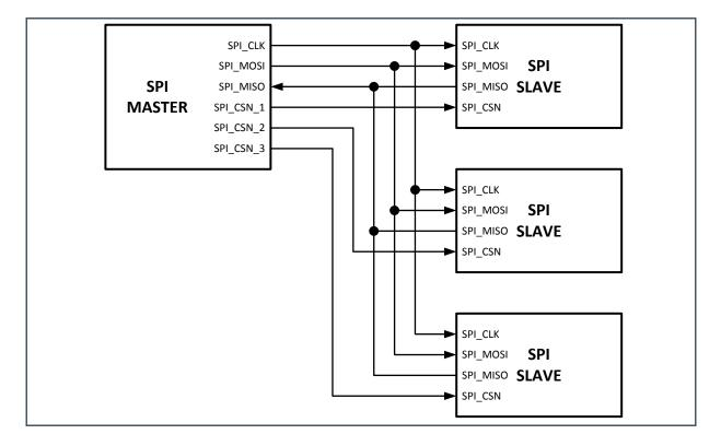
An SPI access always consists of the transfer of the following bits (in this order), as given in Figure 23:
