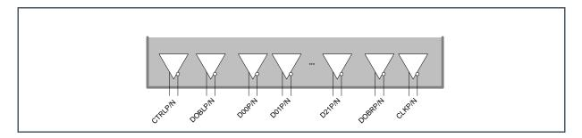
Each pair of differential output pins transports data on one sub-LVDS channel.
