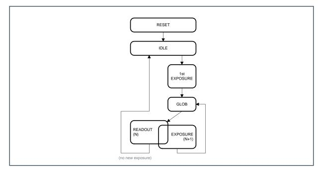
When exiting IDLE state, the first EXPOSURE period starts. Just like in the sequential operation, this flows into a GLOB state, which in its turn starts the READOUT of a frame. Depending on the sensor control or configuration (see 7.2.7 and 7.2.8 for details and options), a new EXPOSURE may start when the READOUT is still busy.
