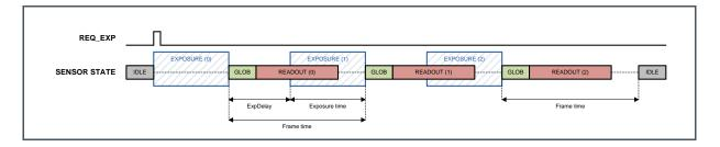
In the example, the programmed 'frame time' is longer than the sum of GLOB length and READOUT length. This situation is allowed and provides an easy mechanism to fine-tune frame rate.
