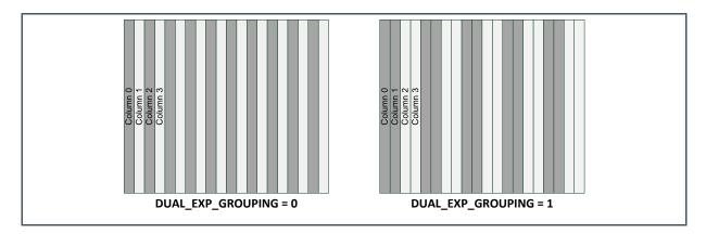
When **DUAL\_EXPOSURE** is set low, the exposure time of all pixels is set with **EXP\_TIME\_L**. When the register is set high, the exposure time of the two groups can be set independently with **EXP\_TIME\_S** and **EXP\_TIME\_L**.
