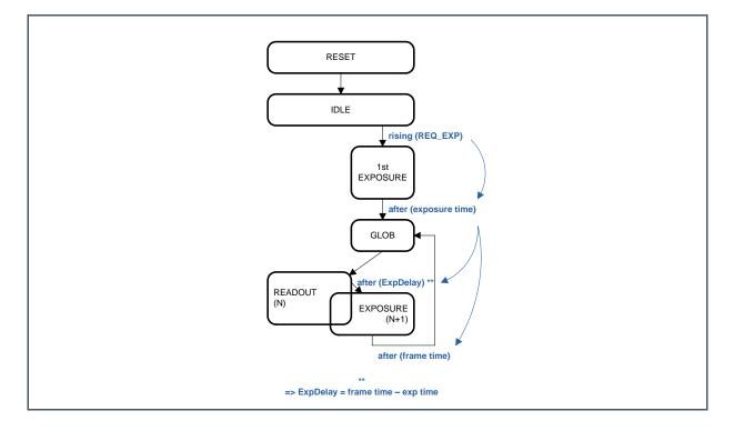
Because of the nature of the streaming mode, there is no such thing as invalid or special control timing. Once started, it will be forever looping and all further REQ\_EXP and REQ\_FRAME pulses are ignored.
