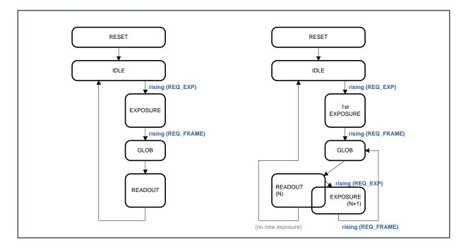
The length of the GLOB state, as well as the length of the READOUT period depends on a number of register settings.
