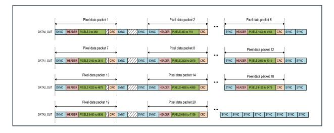
Every used data output channel outputs 6 data packets per line, separated by a number of empty packets.
