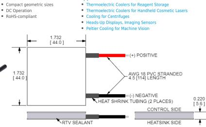
CERAMIC MATERIAL: Al2O3 SOLDER CONSTRUCTION: 138°C. BiSn INCHES [ MM ] Note: Allow 0.020 in [0.5 mm] around perimeter of the thermoelectric cooler and lead wire attachment to accommodate sealant
