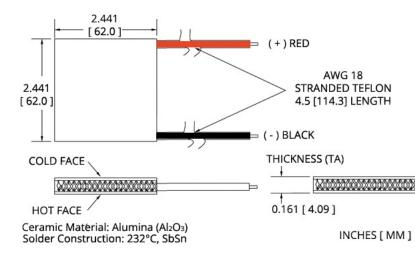
Note: Allow 0.020 in [0.5 mm] around perimeter of the thermoelectric cooler and lead wire attachment to accommodate sealant
