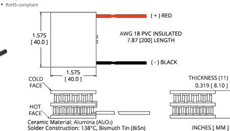
Note: Allow 0.020 in [0.5 mm] around perimeter of the thermoelectric cooler and lead wire attachment to accommodate sealant
