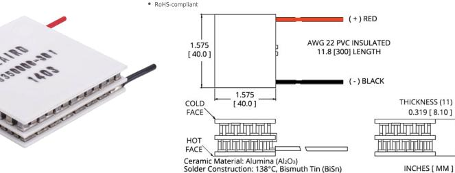
Note: Allow 0.020 in [0.5 mm] around perimeter of the thermoelectric cooler and lead wire attachment to accommodate sealant
