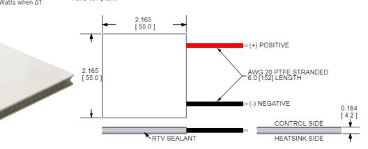
CERAMIC MATERIAL: Al₂O₃ SOLDER CONSTRUCTION: 232°C, SbSn
