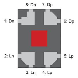
Top View Figure 6.1 Pin Configurations
