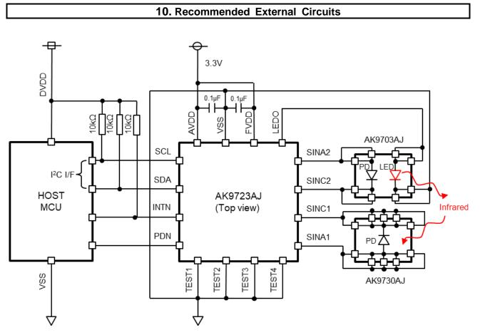
Figure 10.1 Recommended External Circuits
