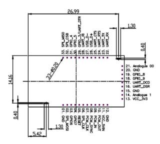
Figure 6-3: BT7xx Mechanical Drawing
