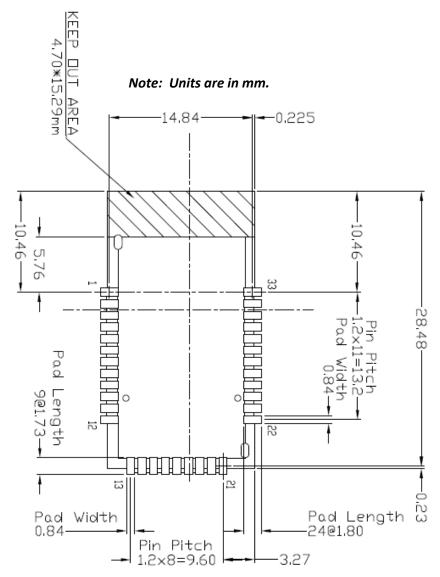
Figure 6-4: PCB Land Pattern and Antenna Keep-out for BT740-SA
