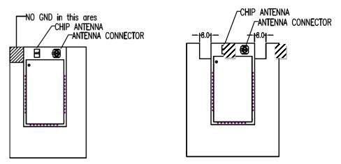
Figure 5-2: BT740-SA placement in the edge (not corner) of host PCB (with modified antenna keep-out).
