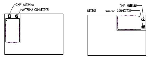
Figure 5-1: BT740-SA placement in the corner of host PCB.
