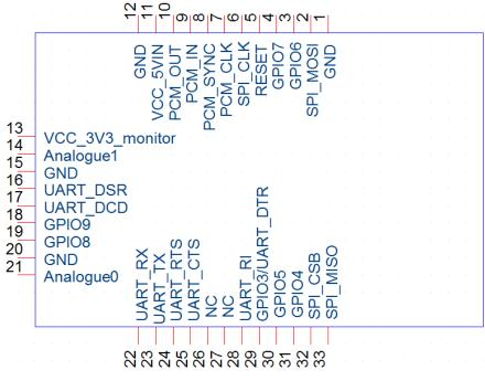
Figure 2-2: BT740-Sx module pin-out (Top View)
