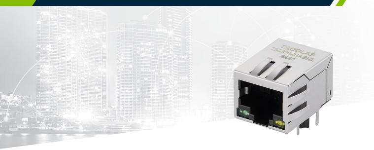
Featuring a popular footprint and compatible package to industry RJ45 Integrated Connectors standards, the Taoglas TMJ0026ABNL is an RJ45 Integrated Connector 10/100Base-T Single Port Tab Down with EMI Finger, its shielded short body design offers extra space, and with a schematic that enables Auto Transformer feature that will provide better EMI performance.
