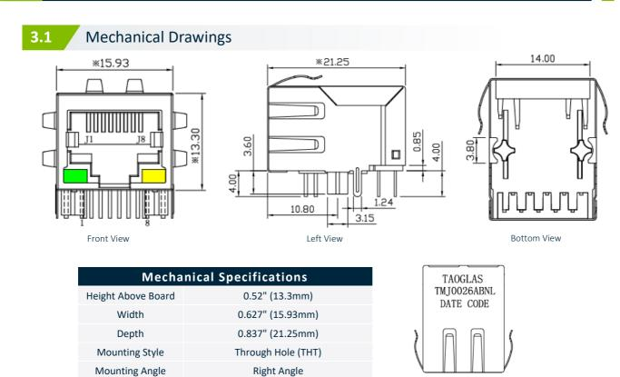
Dimensions are in millimeters with the following tolerances:  $X.XX = \pm 0.25$
