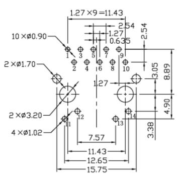
Suggested PCB Layout (Top View) Dimensions are in millimeters with the following tolerances: X.XX =  $\pm 0.10$
