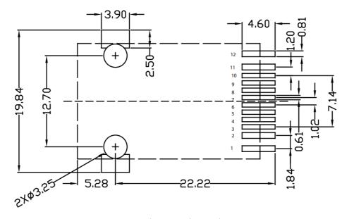
Suggested PCB Layout (Top View) Dimensions are in millimeters with the following tolerances: X.XX =  $\pm 0.10$
