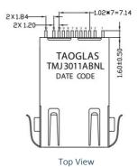
Dimensions are in millimeters with the following tolerances:  $X.XX = \pm 0.25$
