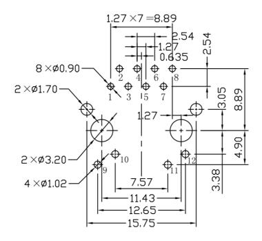
$\label{eq:Suggested} Suggested\ PCB\ Layout\ (Top\ View)$  Dimensions are in millimeters with the following tolerances: X.XX =  $\pm 0.10$
