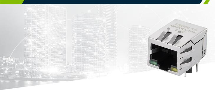
Featuring a popular footprint and compatible package to industry RJ45 Integrated Connectors standards, the Taoglas TMJ4011ABNL is an RJ45 Integrated Connector 10/100Base-T Single Port Tab Down with EMI Finger, its shielded short body design offers extra space, and with a schematic that enables AutoMDIX feature.
