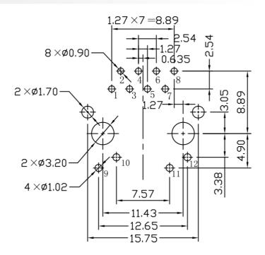
$\label{eq:Suggested PCB Layout (Top View)}$  Dimensions are in millimeters with the following tolerances: X.XX =  $\pm 0.10$
