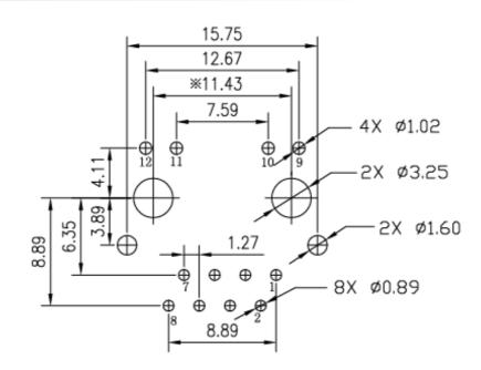
Suggested PCB Layout (Top View) Dimensions are in millimeters with the following tolerances: X.XX =  $\pm 0.10$
