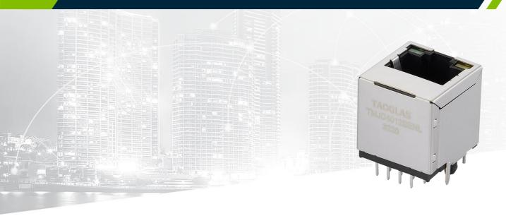
Featuring a popular footprint and compatible package to industry RJ45 Integrated Connectors standards, the Taoglas TMJD4012BENL is an RJ45 Integrated Connector 10/100Base-T Single Port and Vertical with shielded body and with a schematic that enables AutoMDIX feature.
