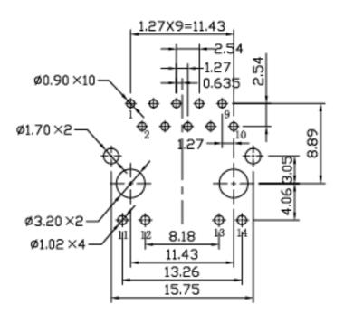
Suggested PCB Layout (Top View) Dimensions are in millimeters with the following tolerances: X.XX =  $\pm 0.10$
